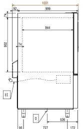
Drain Electrical inlet (power)
